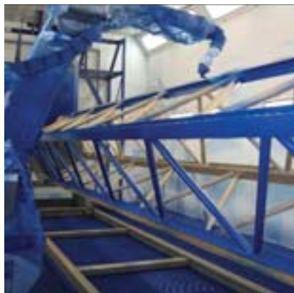
2K waterborne polyurethane applied by automatic spray to crane components.
